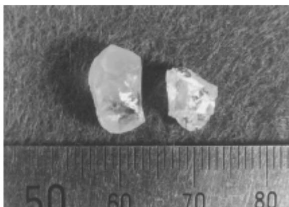
**Figure 1.** Photographs of the crystals grown at the cooling rate of 2 °C/hr.
