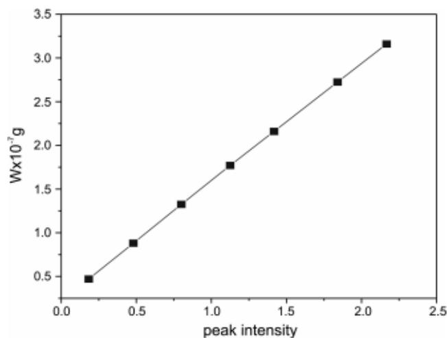
Figure 3. Correlation between the concentration of bisphenol A in solution and the peak intensity in photo-CIDNP.
