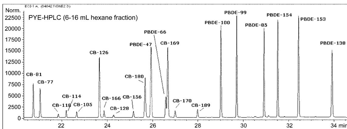
**Figure 3.** A typical chromatogram of PBDE and co-planar PCB elution, in a slightly modified PYE column chromatography GC-micro ECD method. Peaks are identified based on their IUPAC numbers.
