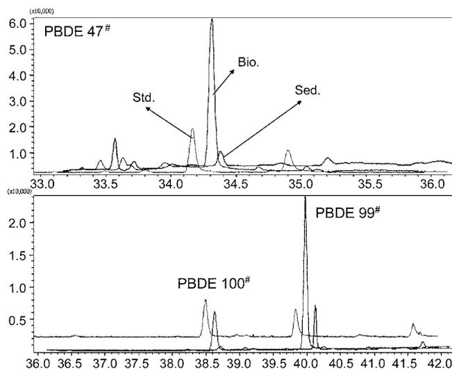
**Figure 5.** GC-MS mass spectrograms of standard, biological tissue and sediment of PBDEs 47, 99 and 100. The chromatograms are slightly displaced for clarity.
