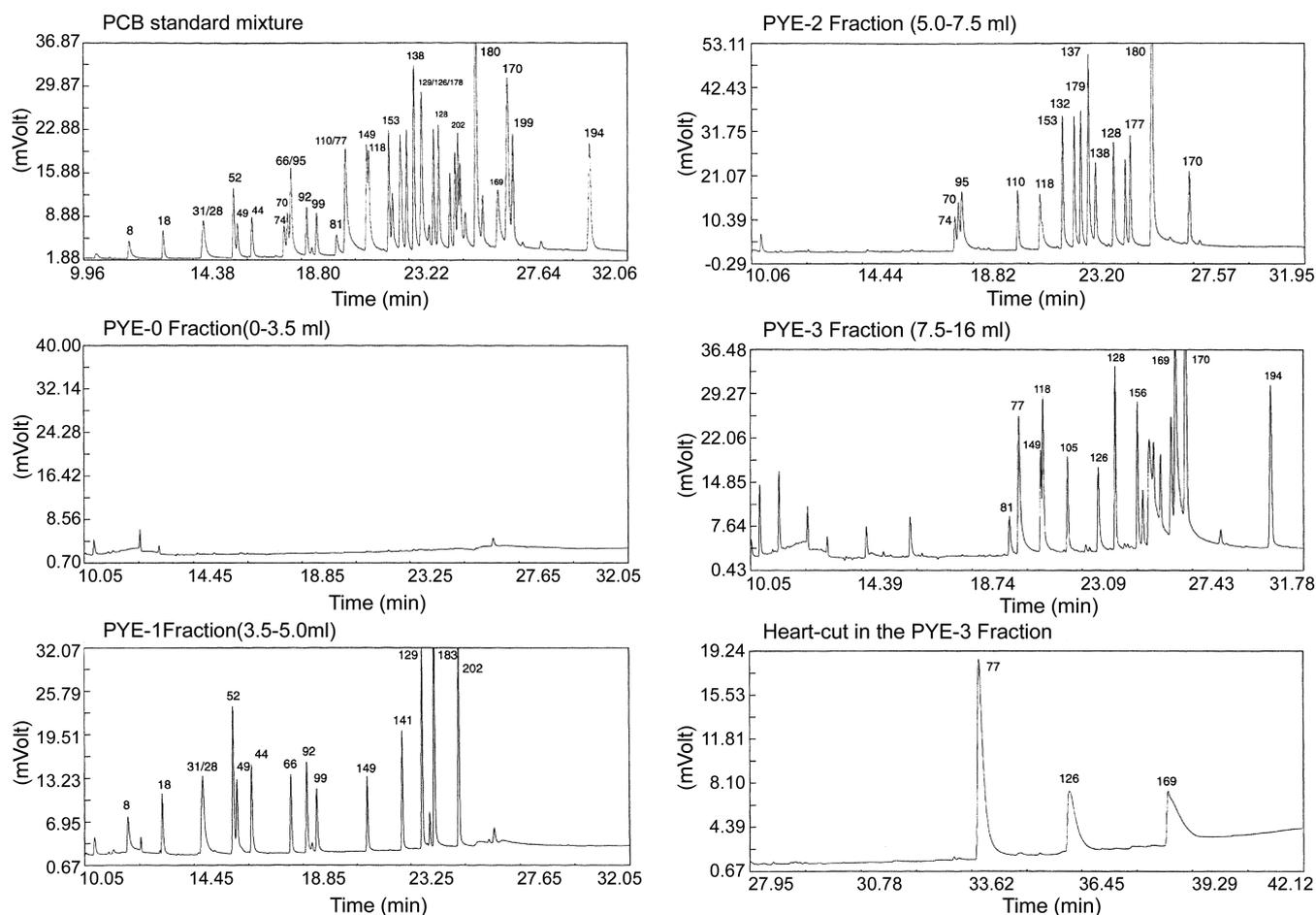
**Figure 1.** GC-ECD chromatograms of a test solution. 0 fraction (0-3.5 mL); 1 fraction (3.5-5.0 mL); 2 fraction (5.0-7.5 mL); 3 fraction (7.5-16 mL) and main ECD chromatogram of a heart-cut for PCBs-77, -126 and -169. No co-elution from PCBs-110, -129 and -178 was noted.
