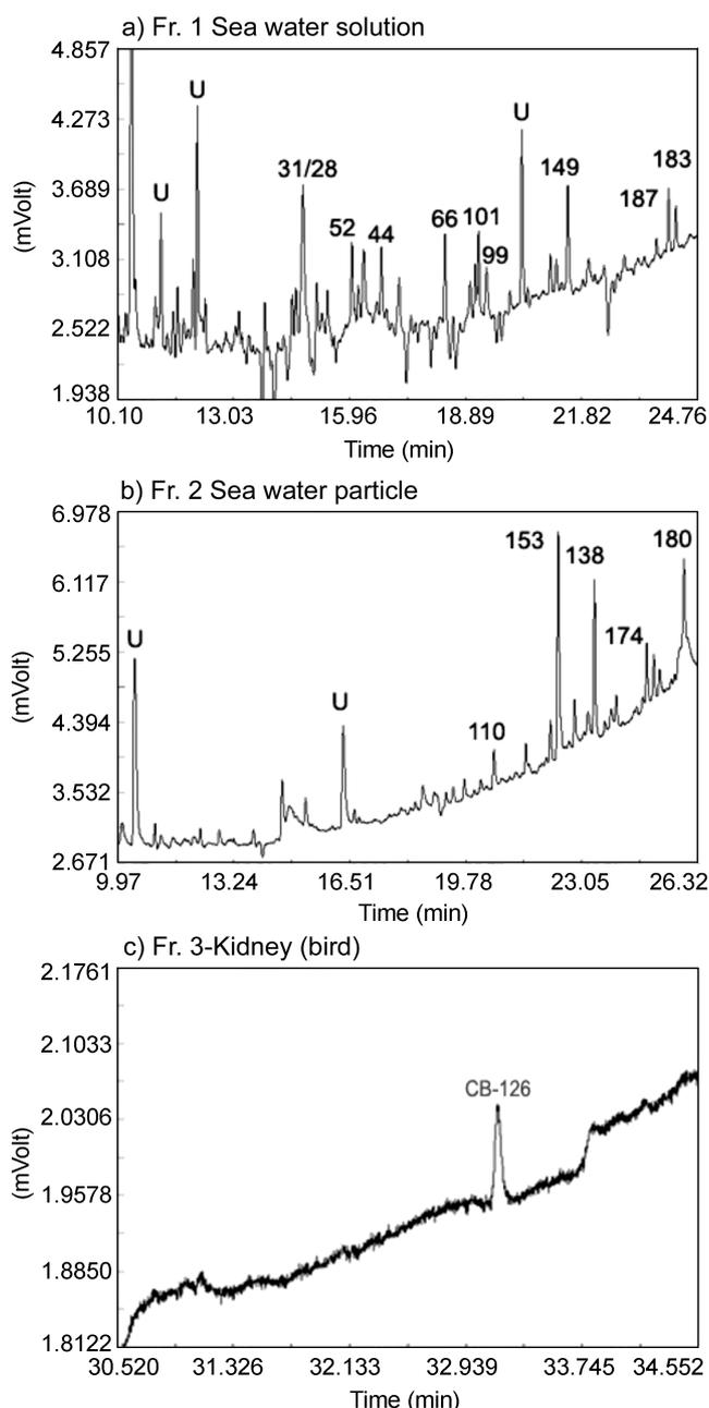
**Figure 2.** GC-ECD chromatograms of environmental samples. Portions from a sensitive range. a) an extract from German coastal water (solution). U-represent non-PCB peaks of unknown environmental origin, b) suspended particulate matter from German coastal zone and, c) chromatogram after a heart-cut of Aoks (Alkan).
