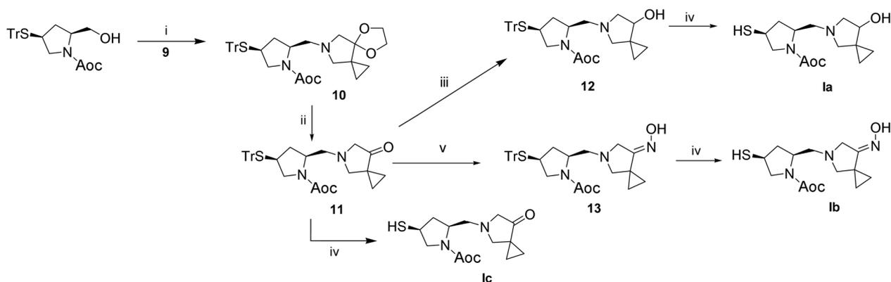
**Scheme 2.** (i) 1. *p*-toluene sulfonyl chloride, TEA,  $CH_2Cl_2$ . 2. **8**, TEA,  $CH_2Cl_2$ . (ii) 1 N-HCl. (iii)  $NaBH_4$ , THF. (iv) trifluoroacetic acid, triethylsilane,  $CH_2Cl_2$ . (v) hydroxylamine hydrochloride, TEA, EtOH.
