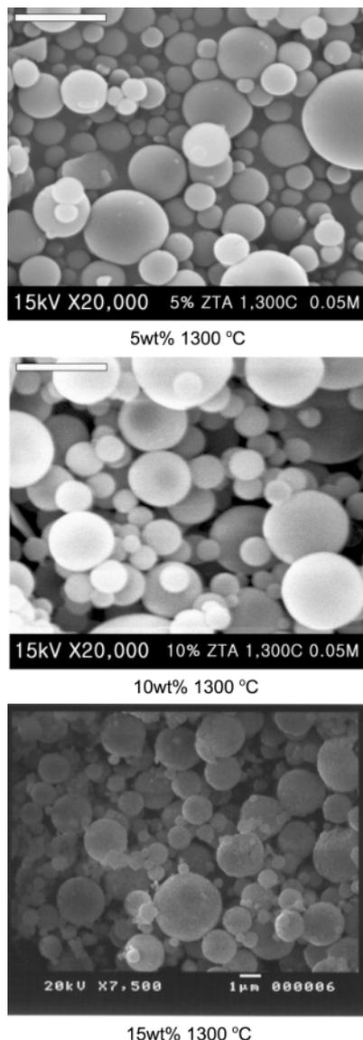
**Figure 3.** SEM photographs of as-prepared ZTA powder by ultrasonic spray pyrolysis at 550 °C drying zone and various temperature of pyrolysis zone with  $\text{Al}(\text{NO}_3)_3 \cdot 9\text{H}_2\text{O}/\text{ZrCl}_2\text{O} \cdot 8\text{H}_2\text{O}$  aqueous solution.
