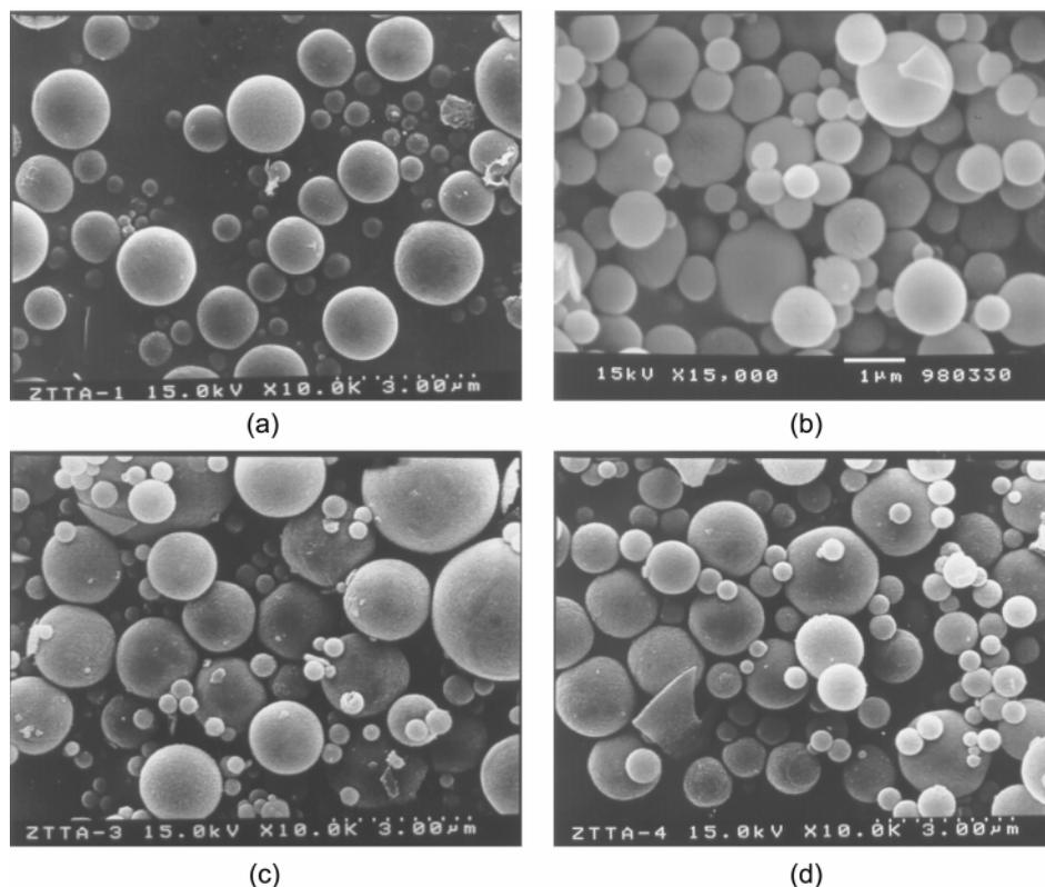
**Figure 8.** SEM photographs of as-prepared ZTTA powder by ultrasonic spray pyrolysis at 500 °C drying zone and 1000 °C temperature of pyrolysis zone with 0.075 M  $\text{Al}(\text{NO}_3)_3 \cdot 9\text{H}_2\text{O} / \text{ZrCl}_2\text{O} \cdot 8\text{H}_2\text{O} / \text{Ti}[\text{OCH}(\text{CH}_3)_2]_4$  aqueous solution. a) ZTTA-1, b) ZTTA-2, c) ZTTA-3, d) ZTTA-4.
