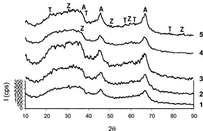
**Figure 7.** X-ray diffraction patterns of as-prepared ZTTA powder by ultrasonic spray pyrolysis at 500 °C drying zone and 1,000 °C pyrolysis zone with 0.05 M mixed aqueous solution. A, Z and T indicate the characteristic peaks of  $\gamma$ -Al<sub>2</sub>O<sub>3</sub>, ZrO<sub>2</sub> and TiO<sub>2</sub> respectively. (1: ZTTA-1, 2: ZTTA-2, 3: ZTTA-3, 4: ZTTA-4, 5: ZTTA-5).
