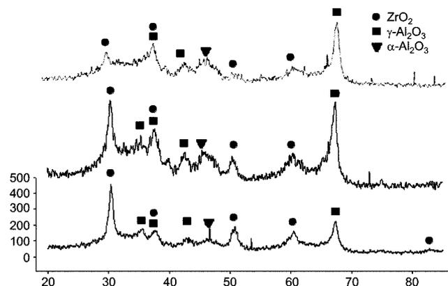
**Figure 2.** X-ray diffraction patterns of as-prepared ZTA powder by ultrasonic spray pyrolysis at 550 °C drying zone and 1200 °C pyrolysis zone with AlCl<sub>3</sub>/ZrCl<sub>2</sub>O · 8H<sub>2</sub>O aqueous solution (bottom: 15 wt%, middle: 10 wt%, top: 5 wt%). ● ZrO<sub>2</sub>, ■ γ-Al<sub>2</sub>O<sub>3</sub>, ▼ α-Al<sub>2</sub>O<sub>3</sub>
