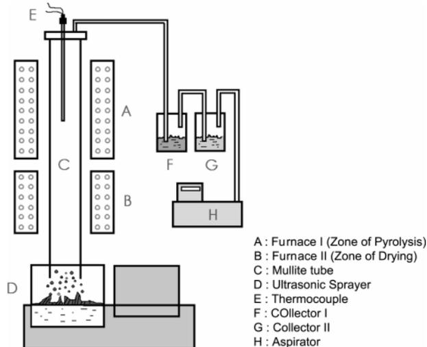
Figure 1. Schematic diagram of ultrasonic spray pyrolysis system.
