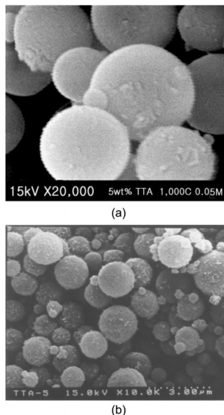
**Figure 4.** SEM photographs of as-prepared TTA powder by ultrasonic spray pyrolysis at 500 °C of drying zone and 1000 °C temperature of pyrolysis zone with  $\text{Al}(\text{NO}_3)_3 \cdot 9\text{H}_2\text{O}/\text{Ti}[\text{OCH}(\text{CH}_3)_2]_4$  aqueous solution. a) 5 wt% TTA powder ( $\times 20,000$ ) b) ( $\times 10,000$ ).
