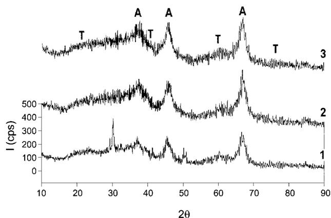
**Figure 6.** X-ray diffraction patterns of as-prepared TTA powder by ultrasonic spray pyrolysis at  $500^\circ\text{C}$  drying zone and  $1,000^\circ\text{C}$  pyrolysis zone with 0.05 M mixed aqueous solution. A and T indicates the characteristic peaks of  $\gamma$ - $\text{Al}_2\text{O}_3$  and  $\text{TiO}_2$  respectively. (1: 2.5 wt% TTA, 2: 5 wt% TTA, 3: 10 wt% TTA)
