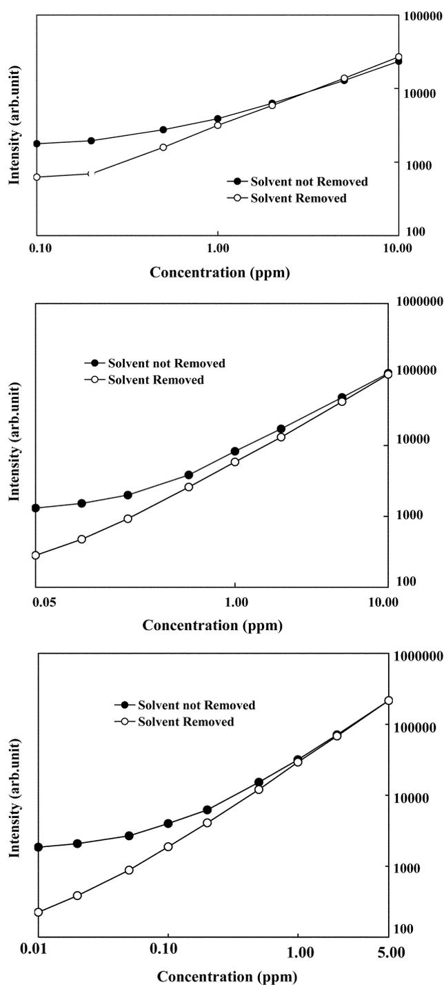
**Figure 7.** (a) Calibration curve of Bi I 306.772 nm for wet (●) and dry (○) plasmas. (b) Calibration curve of Al I 309.271 nm for wet (●) and dry (○) plasmas. (c) Calibration curve of V II 310.230 nm for wet (●) and dry (○) plasmas.
