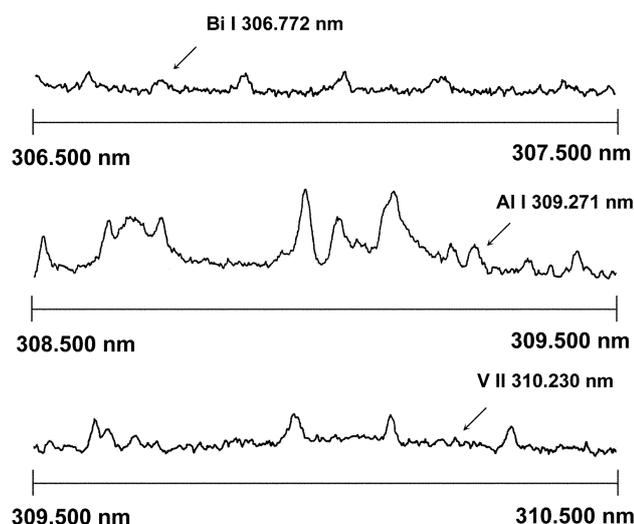
**Figure 4.** OH spectrum over 1.000 nm spectral window for Bi I 306.772 nm, Al I 309.271 nm, V II 310.230 nm for dry plasma using the extended torch. OH interference is completely removed with the use of high tangential gas flow rate and extended torch.
