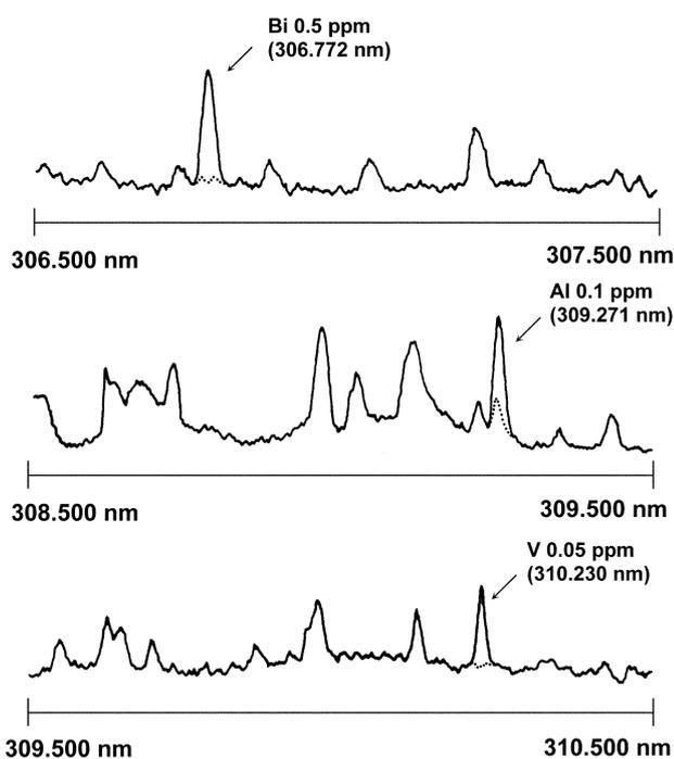
**Figure 6.** Removal of OH interference in wet plasma with Ar cryogenic desolvation system for Bi I 306.772 nm, Al I 309.271 nm, V II 310.230 nm. The dotted lines are OH background. When compared with Figure 4, the Ar cryogenic trap is quite effective in removing OH interferences. Experimental conditions: Extended torch; Outer gas flow rate: 20 L/min.
