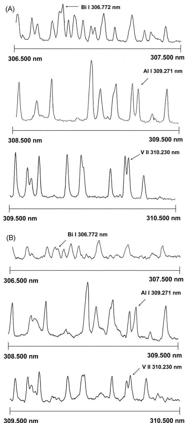
**Figure 2.** (a) OH band interferences on Bi I 306.772 nm, Al I 309.271 nm, V II 310.230 nm with aqueous solvent nebulization. Experimental conditions: Normal torch; Observation height: 15 mm above load coil; Outer gas flow rate: 15 L/min; Sample uptake rate: 1 mL/min. (b) OH band interferences on Bi I 306.772 nm, Al I 309.271 nm, V II 310.230 nm without nebulization. Other experimental conditions are the same as 2-a.
