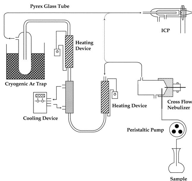
**Figure 1.** Desolvation system used in the experiment. The system is consisted of a condenser, two heater and temperature controllers, and Ar cryogenic trap. The total length of desolvation system is 1.5 m long.
