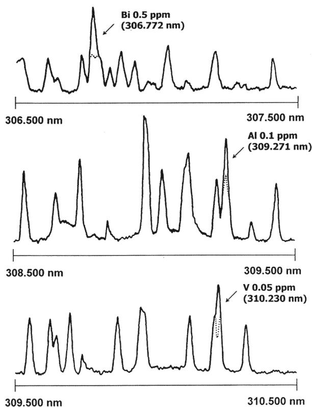
**Figure 5.** Signals and OH band interferences on Bi I 306.772 nm, Al I 309.271 nm, V II 310.230 nm when a condenser is used only. The dotted lines are OH background interferences on analytical lines. Experimental conditions: Extended torch; Outer gas flow rate: 20 L/min.
