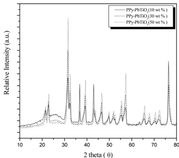
**Figure 2.** XRD patterns of PPy/PbTiO<sub>3</sub> (10 wt %), PPy/PbTiO<sub>3</sub> (30 wt %), and PPy/PbTiO<sub>3</sub> (50 wt %).
