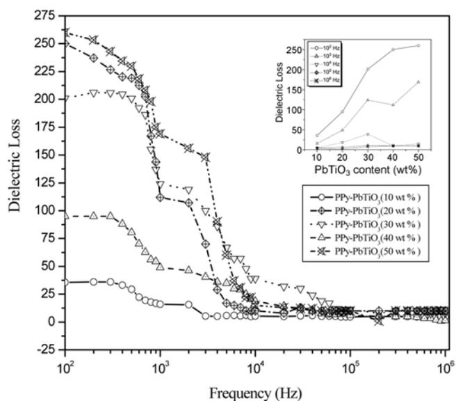
**Figure 7.** Frequency-dependent dielectric loss of  $\text{PPy/PbTiO}_3$  composites (Inset: Dielectric loss of  $\text{PPy/PbTiO}_3$  composites for different wt % of  $\text{PbTiO}_3$  at different frequencies).
