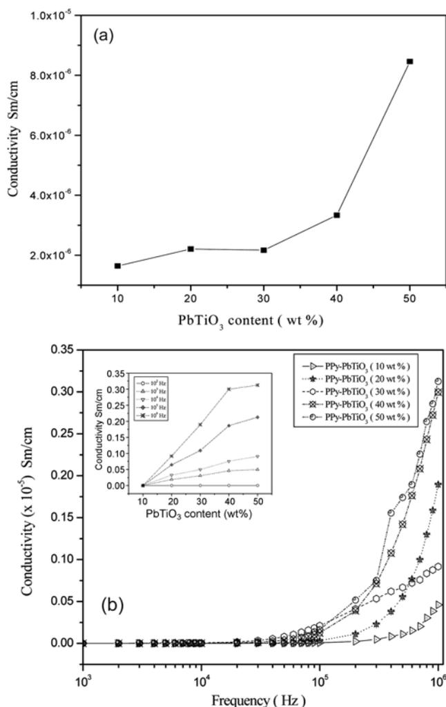
**Figure 5.** Frequency dependence of a.c. conductivity of PPy/PbTiO<sub>3</sub> composites. (a). Variation of conductivity of PPy/PbTiO<sub>3</sub> at different frequency with PbTiO<sub>3</sub> content in the composite (b). At different frequency with increase in the content of PbTiO<sub>3</sub> in the composite (Inset: The conductivity of PPy/PbTiO<sub>3</sub> composites for different wt % of PbTiO<sub>3</sub> at different frequencies).
