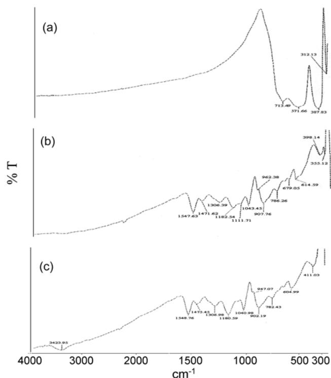
**Figure 1.** FTIR spectra of (a) pure PbTiO<sub>3</sub>, (b) pure PPy, and (c) PPy/PbTiO<sub>3</sub> (30 wt %).
