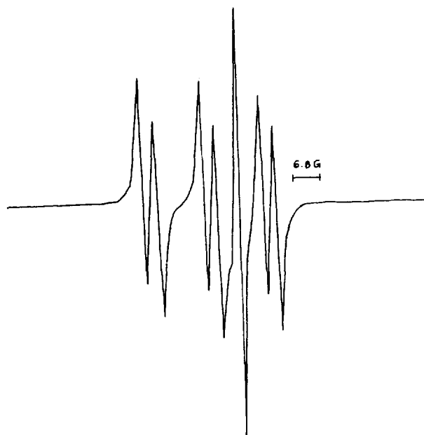
Figure 1. ESR spectrum of the PBN· radical formed in the reaction of ethyl bromide with Li (1% wt. Na) in DBE at r.t. (scanned in 5 min. after mixing.).
