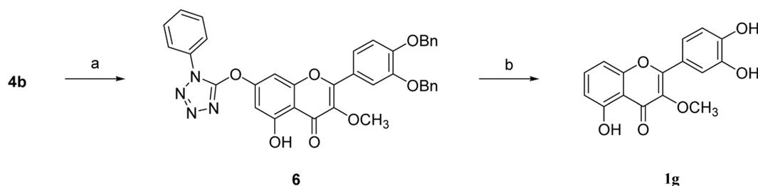
**Scheme 2.** Reagents and conditions: (a) potassium *tert*-butoxide, 5-chloro-1-phenyltetrazole; (b)  $HCOOH$ ,  $Pd/C$ , benzene, EtOH,  $H_2O$ .
