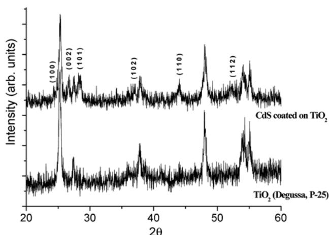
**Figure 2.** XRD patterns for bare  $\text{TiO}_2$  nanoparticles and CdS coated  $\text{TiO}_2$  nanoparticles by sonochemical reaction under MBSL condition.
