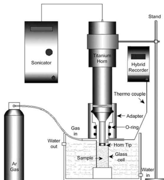
Figure 1. Experimental set-up for MBSL experiment.
