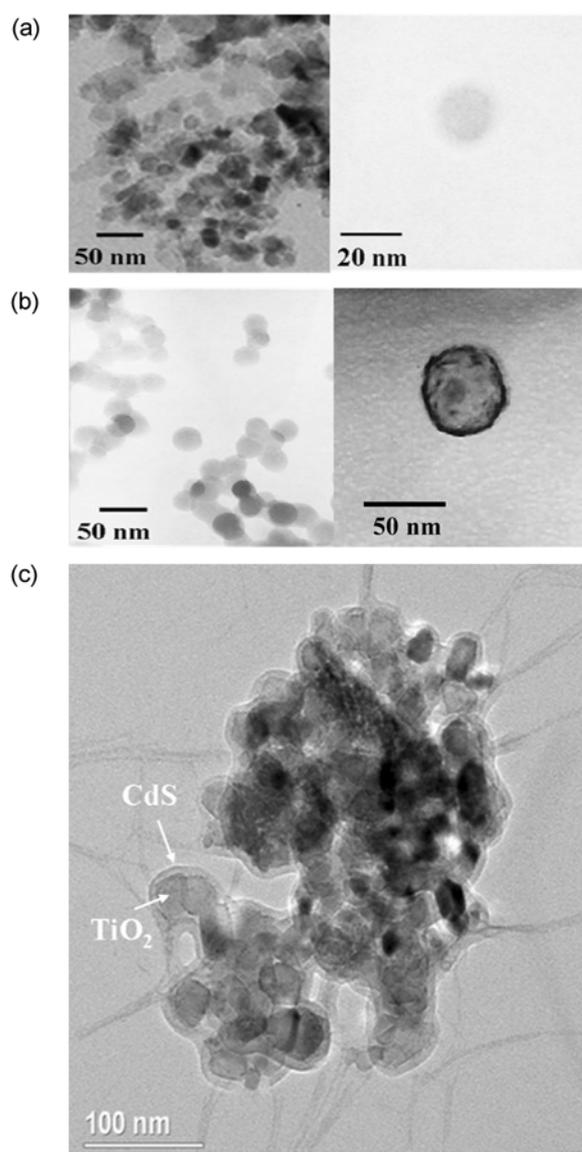
**Figure 4.** Typical TEM images of (a) bare  $\text{TiO}_2$ , (b) CdS-coated  $\text{TiO}_2$  particles, (c) HR-TEM image of CdS-coated  $\text{TiO}_2$  particles prepared under MBSL condition.
