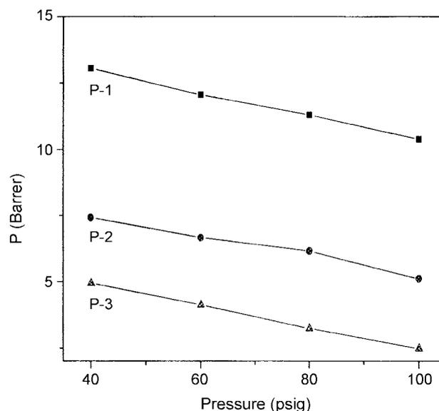
Figure 5.  $P_{\text{O}_2}$  as a function of upstream oxygen gas pressure.
