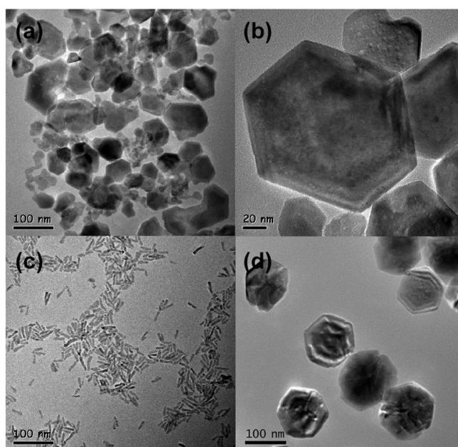
**Figure 3.** (a) The TEM image presents the hexagonal plate shapes of ZnO nanoparticles prepared by Method II. (b) The magnified TEM image (Method II) presents a clear view of the hexagonal shapes of ZnO nanoparticles. (c) The TEM image presents the nanorod shapes of ZnO nanoparticles prepared by Method III. (d) The TEM image presents the hexagonal cone shapes of ZnO nanoparticles prepared by Method I.
