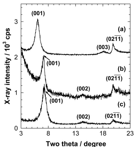
**Figure 1.** Powder XRD patterns of (a) the nickel-intercalated montmorillonite and (b) its derivative calcined at 200 °C, in comparison with that of (c) the pristine Na-montmorillonite.
