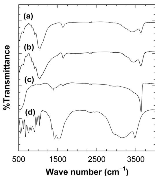
**Figure 7.** FT-IR spectra of (a) the nickel-intercalated montmorillonite, (b) the pristine Na-montmorillonite, (c) Ni(OH)<sub>2</sub>, and (d) Ni(CH<sub>3</sub>COO)<sub>2</sub>.
