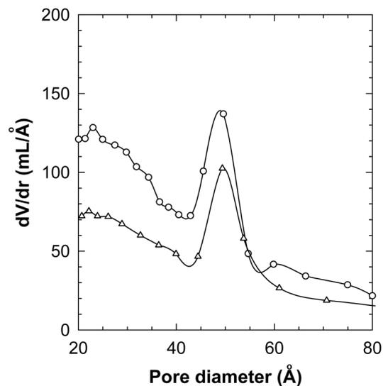
**Figure 5.** Pore size distribution curve for the nickel-intercalated montmorillonite (circles) and its derivative calcined at 200 °C (triangles) analyzed by BJH method.
