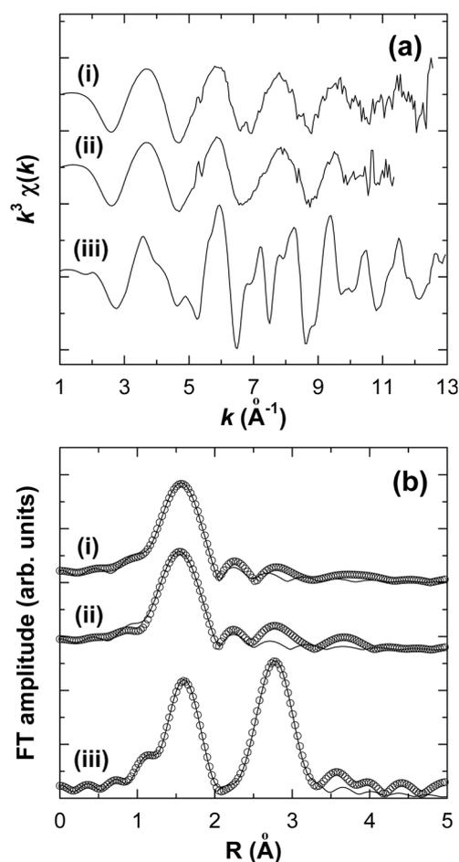
**Figure 9.** (a)  $k^3$ -weighted Ni K-edge EXAFS oscillations and (b) the Fourier-transformed spectra for (i) the as-prepared nickel-intercalated montmorillonite, (ii) its derivative calcined at 200 °C, and (iii) Ni(OH)<sub>2</sub>. The open circles and the solid lines represent the experimental data and the calculated ones, respectively.
