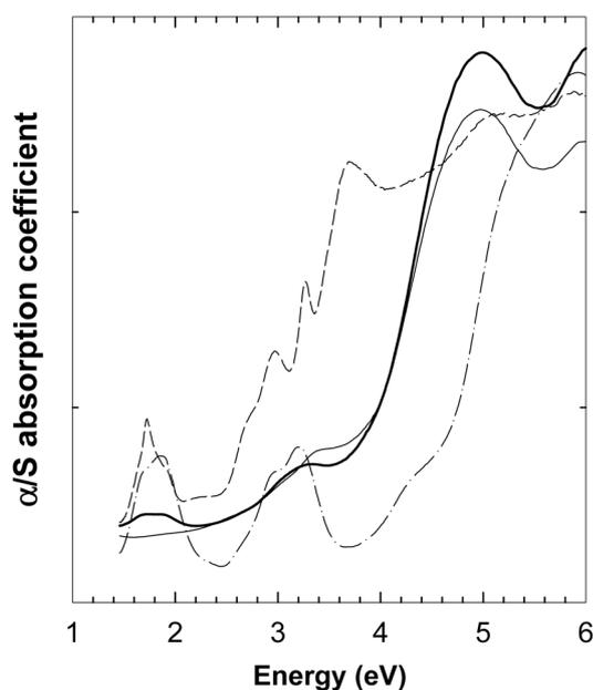
**Figure 6.** Diffuse reflectance UV-vis absorption spectra for the nickel-intercalated montmorillonite (thick solid lines), the pristine Na-montmorillonite (thin solid lines), NiO (dashed lines), and Ni(OH)<sub>2</sub> (dot-dashed lines).
