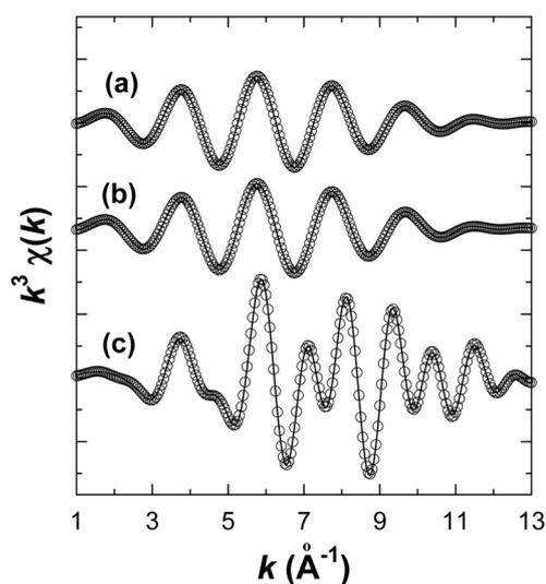
**Figure 10.** Fourier-filtered Ni K-edge EXAFS data for (a) the as-prepared nickel-intercalated montmorillonite, (b) its derivative calcined at 200 °C, and (c) Ni(OH)<sub>2</sub>. The open circles and the solid lines represent the experimental data and the calculated ones, respectively.
