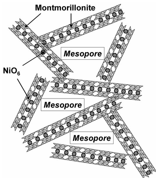
**Figure 11.** Schematic illustration of the nickel-intercalated montmorillonite.
