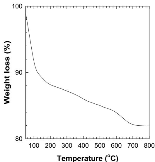
**Figure 2.** TGA curve of the nickel-intercalated montmorillonite under Ar atmosphere.
