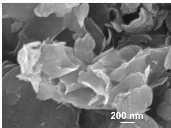
**Figure 3.** FE-SEM image of the nickel-intercalated montmorillonite.
