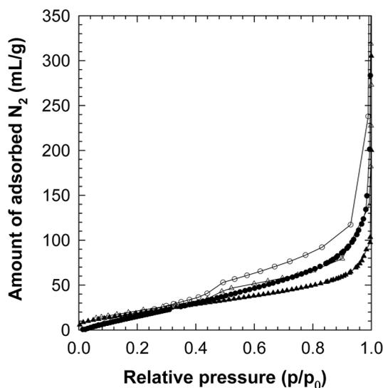
**Figure 4.** N<sub>2</sub> adsorption-desorption isotherms for the nickel-intercalated montmorillonite (circles) and its derivative calcined at 200 °C (triangles).
