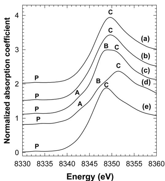
**Figure 8.** Ni K-edge XANES spectra for (a) the nickel-intercalated montmorillonite and (b) its derivative calcined at 200 °C, in comparison with those for the references (c) Ni(OH)<sub>2</sub>, (d) NiO, and (e) Ni(CH<sub>3</sub>COO)<sub>2</sub>.
