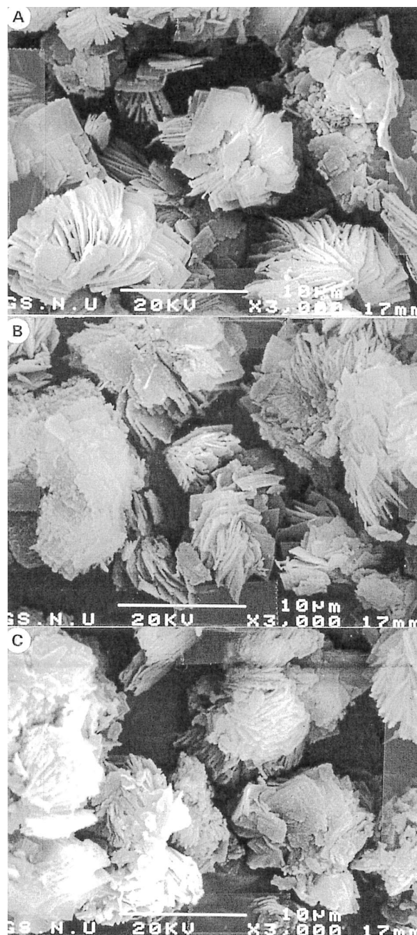
Figure 8. The scanning electron micrographs for the calcined silica-pillared H-kenyaite, hydrolyzed for 10 (A), 20 (B) and 40 (A) min in 0.05 %NH 3 solution.
