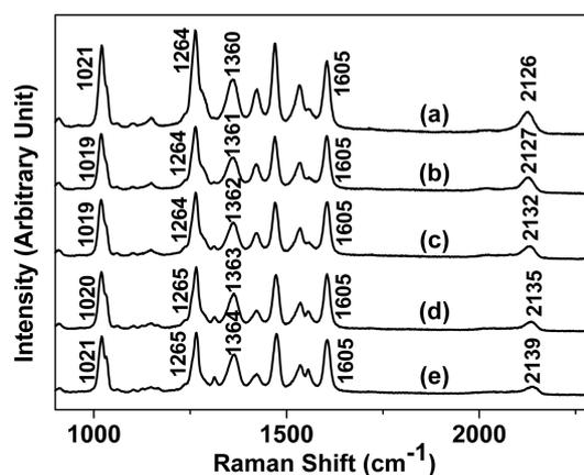
**Figure 5.** SERS spectra of  $\sim 10^{-3}$  M N719 on Ag electrode at various voltages of (a)  $-0.8$ , (b)  $-0.6$ , (c)  $-0.4$ , (d)  $-0.2$ , and (e)  $0.0$  V vs. the standard Ag/AgCl electrode.
