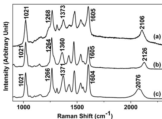
**Figure 3.** SERS spectra of  $\sim 10^{-3}$  M N719 on (a) Au, (b) Ag, and (c) Cu electrode surfaces at a voltage of  $-0.8$  V vs. the standard Ag/AgCl electrode in  $900\text{--}2300\text{ cm}^{-1}$ . All the spectra were taken by the irradiation light source at  $632.8\text{ nm}$  from the HeNe laser.
