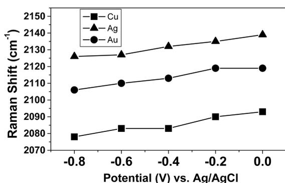
**Figure 7.** Frequency positions of the NCS stretching modes at  $\sim 2100$   $\text{cm}^{-1}$  in the SERS spectra on Cu ( $\blacksquare$ ), Ag ( $\blacktriangle$ ), and Au ( $\bullet$ ) electrode surfaces at various voltages from  $-0.8$  to  $0.4$  V.
