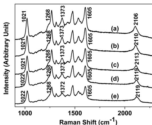
**Figure 4.** SERS spectra of  $\sim 10^{-3}$  M N719 on Au electrode at various voltages of (a)  $-0.8$ , (b)  $-0.6$ , (c)  $-0.4$ , (d)  $-0.2$ , and (e)  $0.0$  V vs. the standard Ag/AgCl electrode.
