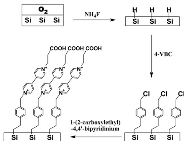
**Scheme 1.** The synthetic sequence of Si(111)-4-vinylbenzyl-1-(2-carboxylethyl)-4,4'-bipyridium.
