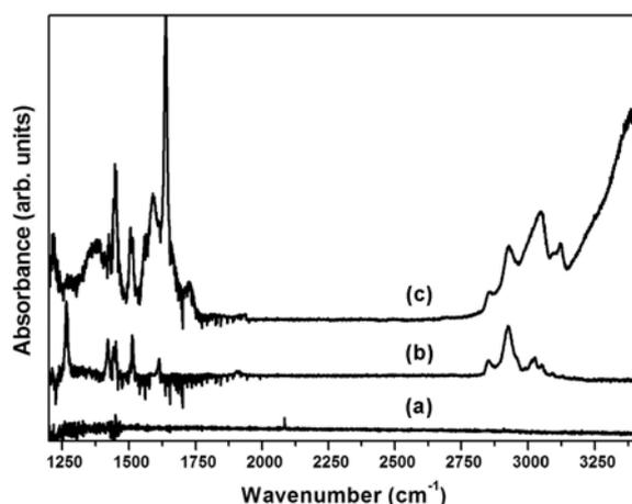
**Figure 1.** ATR-FTIR spectra of (a) H-Si(111), (b) 4-VBC-Si(111), and (c) Si-4-VB-VCOOH substrates.
