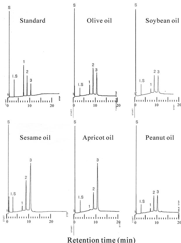
**Figure 1.** Separation of intact triacylglycerols in selected vegetable oils by high temperature gas chromatography with flame ionization detector. (S: solvent, I.S.: internal standard (T<sub>42</sub>), 1: T<sub>50</sub>, 2: T<sub>52</sub>, 3: T<sub>54</sub>)
