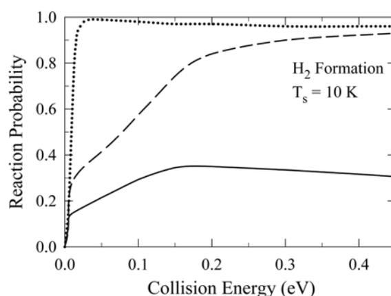
**Figure 10.** Comparison of the probability of  $\text{H}_2(\text{g})$  formation on the collision energy. The solid curve is the present model. The dashed curve is the  $b = 0$  case of the present model. The dotted curve is reproduced from Ref. 18; a smooth curve is taken from the highly oscillatory data.
