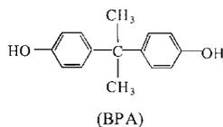
Bis-GMA is a methacrylic ester based on bisphenol-A (BPA), which is the most commonly used matrix material for dental polymers because of its acceptable chemical stability, mechanical properties and ability to simulate natural
