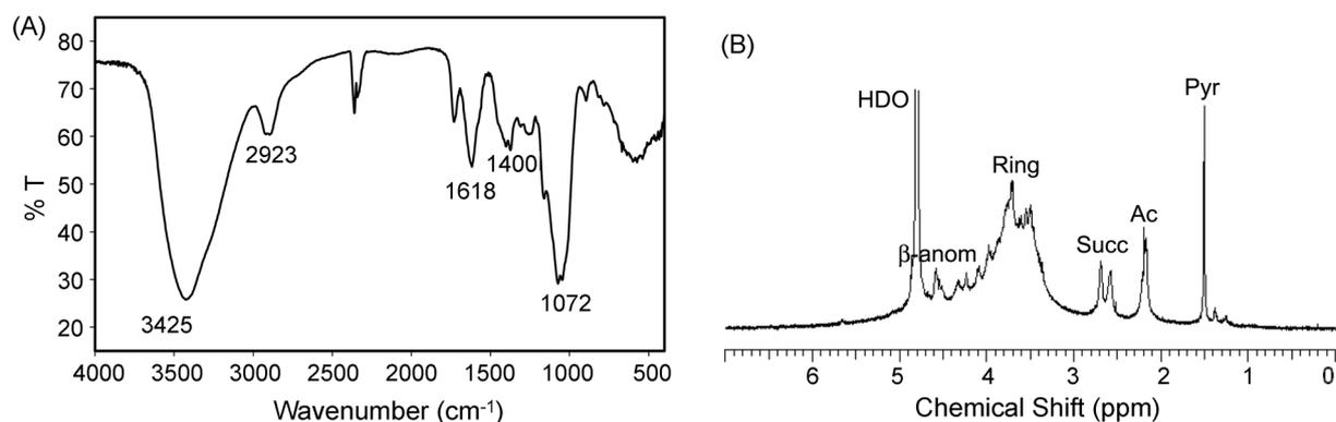
**Figure 2.** Structural identification of succinoglycan isolated from *R. meliloti* 1021. (A) The FT-IR spectrum of succinoglycan. (B)  $^1\text{H}$  NMR spectrum of succinoglycan.  $\beta$ -anom,  $\beta$ -anomeric protons; ring, ring protons of the sugars; succ, methyl protons of the succinyl groups; ac, methyl protons of the acetyl groups; pyr, methyl protons of the 1-carboxyethylidene (pyruvate) groups.
