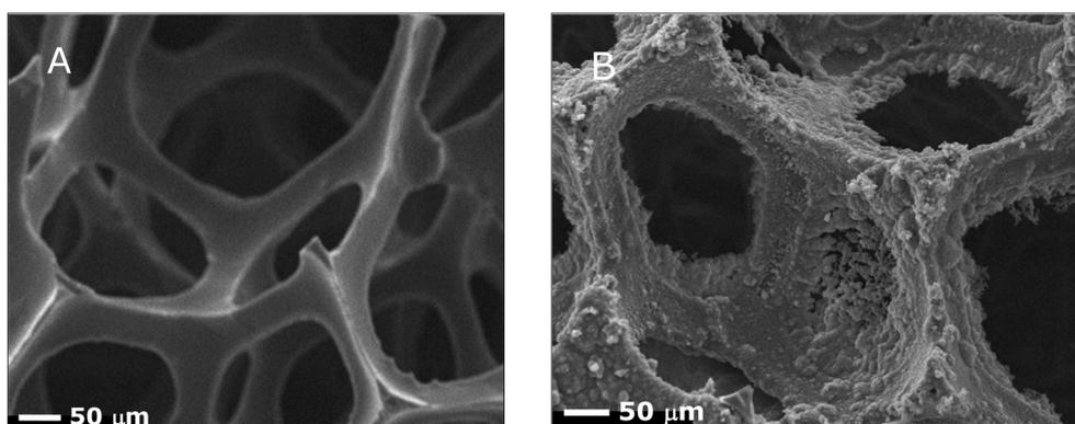
**Figure 1.** SEM images of RVC before (A) and after (B) electropolymerization of pyrrole for 15 min.
