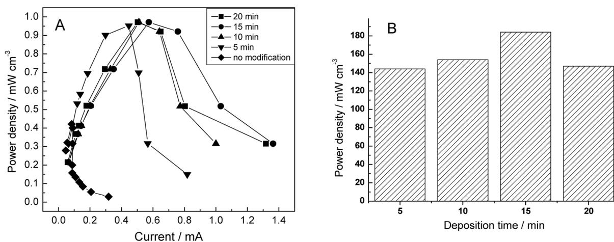
**Figure 2.** Polarization curves (A) and power density vs deposition time (B) for a MFC comprised of *P. vulgaris* (80 mg mL<sup>-1</sup>), methylene Blue (0.5 mM), and glucose (0.01 M) for different deposition time of 0 (♦), 5 (▼), 10 (▲), 15 (●), and 20 min (■). The solutions were buffered at pH 7.0.
