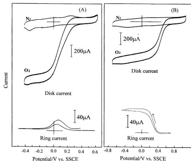
**Figure 4.** RRDE currents with oxygen reduction at PEDT-MTSP disk electrodes in  $O_2$ -saturated 0.05 M  $H_2SO_4$ . (A) PEDT-FeTSP, (B) PEDT-CoTSP. Scan rate:  $50 \text{ mV s}^{-1}$ ; Rotation rate: 2000 rpm.
