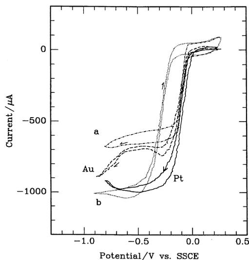
**Figure 3.**  $\text{O}_2$  reduction currents at rotating PEDT-CoTSP (a), PEDT-FeTSP (b), Pt, and Au electrodes in  $\text{O}_2$ -saturated 0.1 M KOH. Scan rate:  $50 \text{ mV s}^{-1}$ ; Rotation rate: 2000 rpm; Electrode area:  $0.164 \text{ cm}^2$ .
