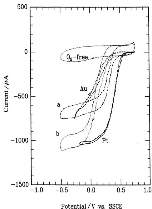
**Figure 2.**  $\text{O}_2$  reduction currents at rotating PEDT-CoTSP (a), PEDT-FeTSP (b), Pt, and Au electrodes in  $\text{O}_2$ -saturated 0.05 M  $\text{H}_2\text{SO}_4$ . Scan rate:  $50 \text{ mV s}^{-1}$ ; Rotation rate: 2000 rpm; Electrode area:  $0.164 \text{ cm}^2$ .
