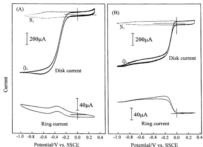
**Figure 5.** RRDE currents with oxygen reduction at PEDT-MTSP disk electrodes in  $O_2$ -satd. 0.1 M KOH. (A) PEDT-FeTSP, (B) PEDT-CoTSP. Scan rate:  $50 \text{ mV s}^{-1}$ ; Rotation rate: 2000 rpm.
