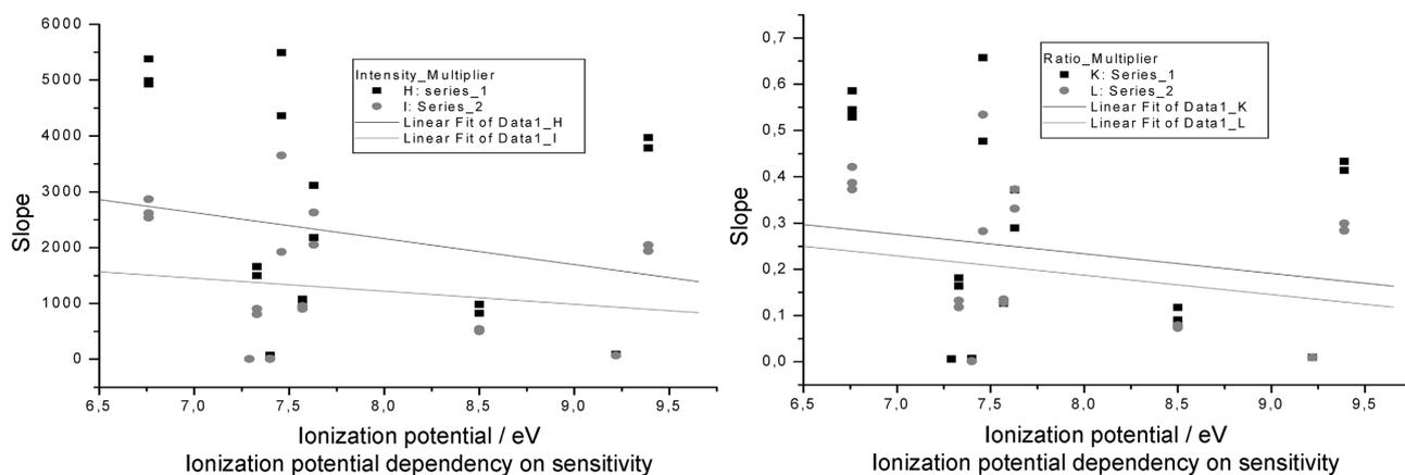
Figure 6. Dependence of an ionization potential on the variation of the sensitivity factor of element by GD-MS.
