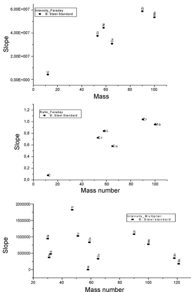
Figure 7. Mass dependence on sensitivity factor in steel standards by GD-MS.
