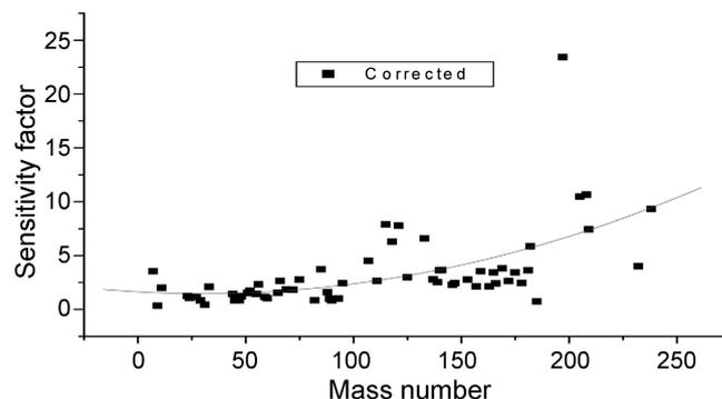
**Figure 3.** Sensitivity factors of elements in glass type specimen by a laser ablation ICP-MS.
