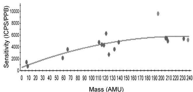
**Figure 2.** Sensitivity factors of elements in liquid solution by ICP-MS.
