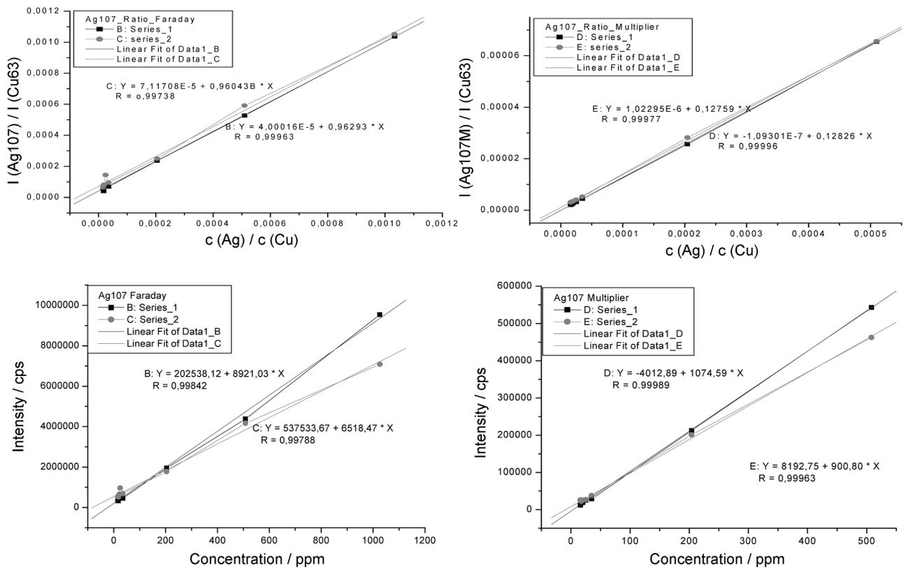
Figure 4. GD-MS calibration curves of Ag107 in copper standards by the Faraday cup detector and the electron multiplier detector.
