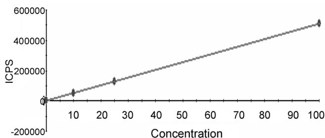
**Figure 1.** Calibration curve of U238 in liquid solution by a laser ablation ICP-MS.
