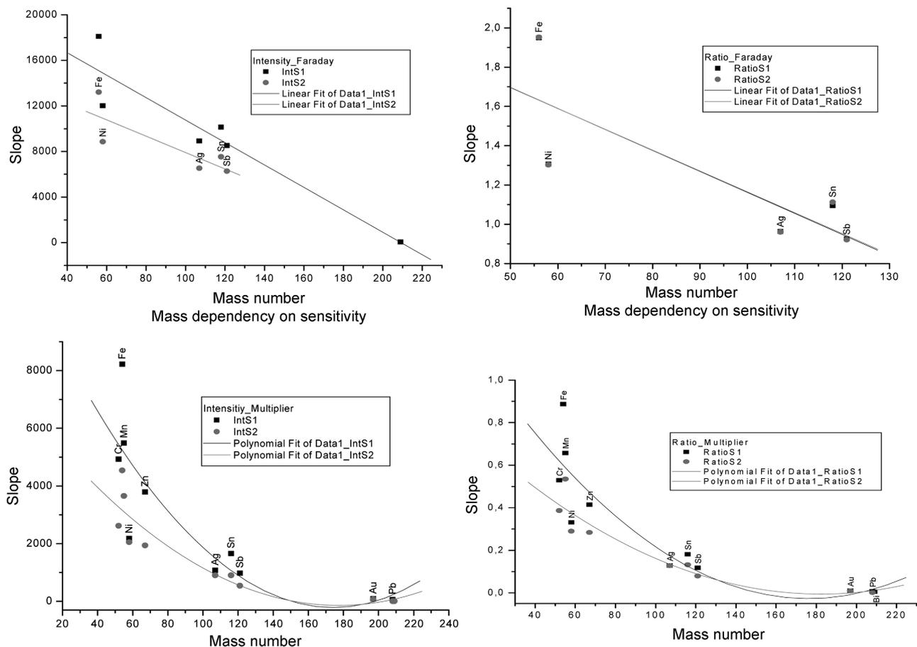
Figure 5. Mass dependence on sensitivity factor in Cu standards by GD-MS.
