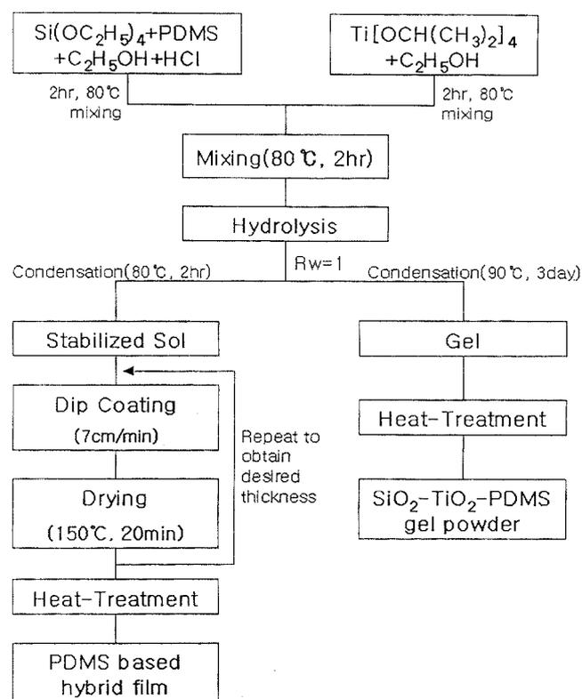
**Figure 1.** Flow diagram for the preparation of SiO<sub>2</sub>-TiO<sub>2</sub>-PDMS thin film and powder.
