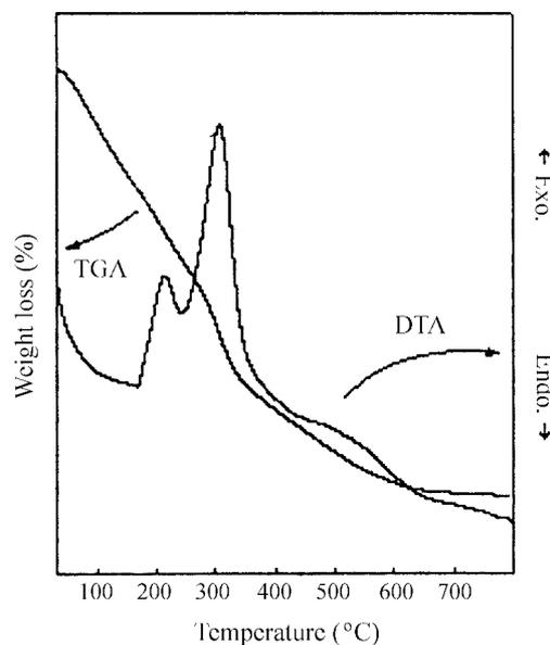
**Figure 2.** (a) TGA and (b) DTA of SiO<sub>2</sub>-TiO<sub>2</sub>-PDMS powder.
