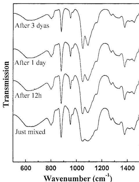
Figure 4. FT-IR spectra during the hydrolysis of SiO<sub>2</sub>-TiO<sub>2</sub>-PDMS sols.
