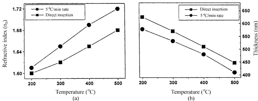
**Figure 8.** Refractive Index (a) and Film Thickness (b) of  $70\text{SiO}_2\text{-}30\text{TiO}_2\text{-}5$  wt.% PDMS thin films heat-treated at various temperatures for 30 min with different heating rate.
