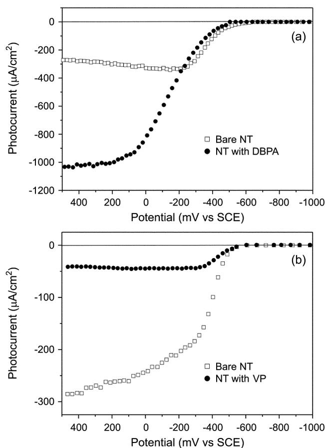
**Figure 2.** Photocurrent-potential characteristics of (a) DBPA-adsorbed and (b) VP-adsorbed NT electrode compared with that of bare NT electrode in 0.1 M KCl solution (light intensity:  $166 \text{ mW/cm}^2$ , wavelength  $>330 \text{ nm}$ )
