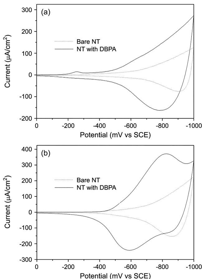
**Figure 1.** Cyclic voltammograms of (a) DBPA-adsorbed and (b) VP-adsorbed NT electrode compared with that of bare NT electrode in 0.1 M KCl solution. (scan rate: 20 mV/s)
