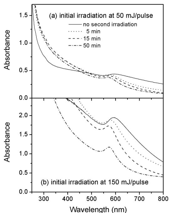
**Figure 3.** Optical absorption spectra of the Cu nanoparticles prepared in 2-propanol by 532 nm laser ablation at various irradiation condition. Solid lines denote the absorption spectra after only initial irradiation at 50 mJ/pulse (panel a) and 150 mJ/pulse (panel b) for 30 min. Broken lines denote the absorption spectra after the second stage irradiation at 250 mJ/pulse for 5 min (dotted line), 15 min (dashed line), and 50 min (dash-dotted line).
