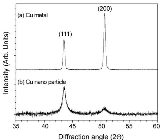
**Figure 2.** X-ray diffraction profiles of dried suspensions obtained by laser ablation of Cu powder dispersed in 2-propanol.
