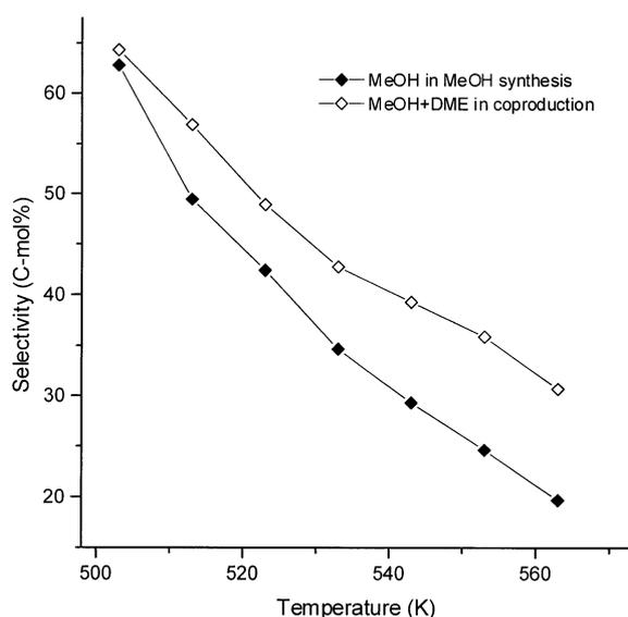
**Figure 3.** Comparison of oxygenate selectivity between methanol synthesis and MeOH+DME co-production: pressure = 3 MPa; catalyst (CuO/ZnO/Al<sub>2</sub>O<sub>3</sub>; silica-alumina) hybrid = 1 : 1 wt. ratio; contact time = 0.125 s · g/mL (contact time is based on only CuO/ZnO/Al<sub>2</sub>O<sub>3</sub>).
