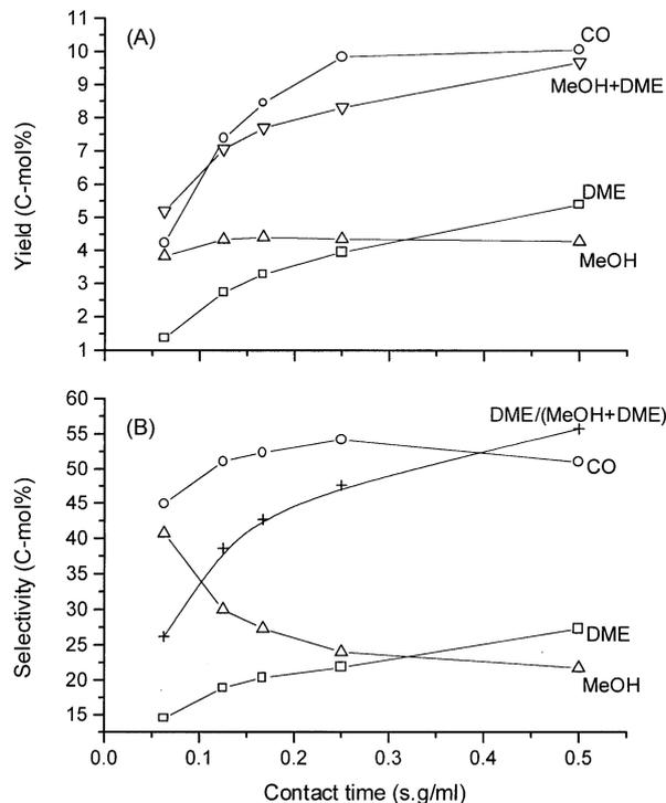
**Figure 5.** Dependence of yields and selectivities on contact time in MeOH+DME co-production (contact time is based on only CuO/ZnO/Al<sub>2</sub>O<sub>3</sub>): pressure = 3 MPa; catalyst (CuO/ZnO/Al<sub>2</sub>O<sub>3</sub>: silica-alumina) hybrid = 1 : 1 wt. ratio; reaction temperature = 523 K.
