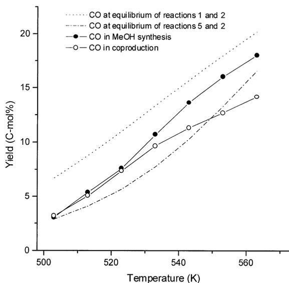
**Figure 2.** Comparison of CO yield between methanol synthesis and MeOH+DME co-production: pressure = 3 MPa; catalyst (CuO/ZnO/Al<sub>2</sub>O<sub>3</sub>; silica-alumina) hybrid = 1 : 1 wt. ratio; contact time = 0.125 s · g/mL (contact time is based on only CuO/ZnO/Al<sub>2</sub>O<sub>3</sub>).
