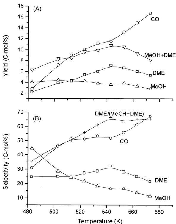
**Figure 4.** Dependence of yields and selectivities on reaction temperature in MeOH+DME co-production: pressure = 3 MPa; catalyst (CuO/ZnO/Al<sub>2</sub>O<sub>3</sub>: silica-alumina) hybrid = 1 : 1 wt. ratio; contact time = 0.5 s · g/mL (contact time is based on only CuO/ZnO/Al<sub>2</sub>O<sub>3</sub>).
