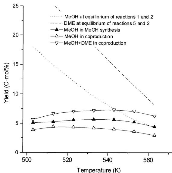
**Figure 1.** Comparison of oxygenate yields between methanol synthesis and MeOH+DME co-production: pressure = 3 MPa; catalyst ( $\text{CuO}/\text{ZnO}/\text{Al}_2\text{O}_3$ : silica-alumina) hybrid = 1 : 1 wt. ratio; contact time = 0.125 s  $\cdot$  g/mL (contact time is based on only  $\text{CuO}/\text{ZnO}/\text{Al}_2\text{O}_3$ ).
