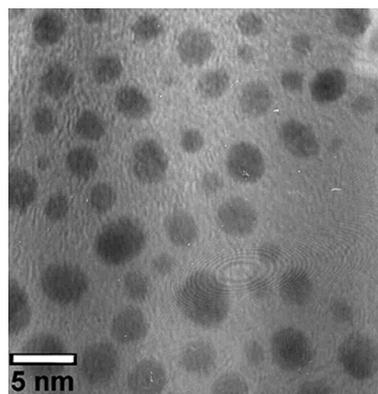
**Figure 2.** TEM image of the undecanethiol-coated gold nanoparticles.
