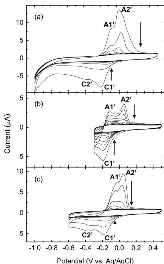
**Figure 7.** Ten consecutive cyclic voltammograms of BpCu-coated GCE in 0.1 M acetate buffer (pH 4.7) saturated with Ar with a negative potential limit of (a)  $-1.0 \text{ V}$ , (b)  $-0.3 \text{ V}$ , and (c)  $-0.6 \text{ V}$ . Scan rate =  $100 \text{ mV} \cdot \text{s}^{-1}$ .
