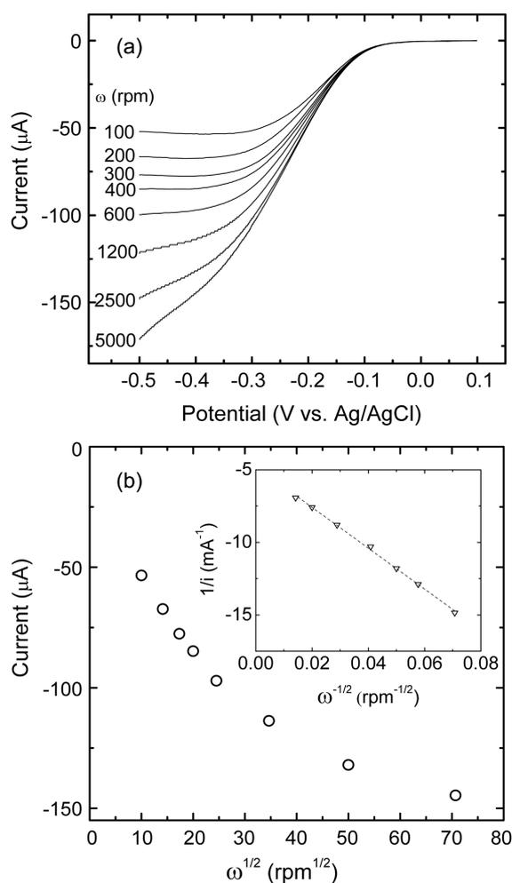
**Figure 5.** (a) RDE voltammograms of pBpCuOx-coated GCE in 0.1 M acetate buffer saturated with O<sub>2</sub> at various rotation rates. Scan rate = 25 mV·s<sup>-1</sup>. (b) Plot of the current at -0.4 V as a function of the square root of the rotation rate. The inset is Koutechy-Levich plot obtained from the RDE voltammograms in Figure 5a at -0.4 V.
