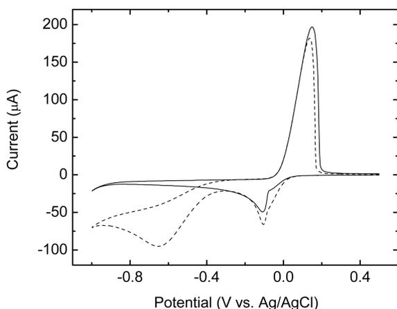
**Figure 6.** Cyclic voltammograms of a bare GCE in 1 mM  $CuCl_2 + 0.1 \text{ M}$  acetate buffer (pH 4.7) saturated with Ar (solid line) and  $O_2$  (dashed line). Scan rate =  $100 \text{ mV} \cdot \text{s}^{-1}$ .
