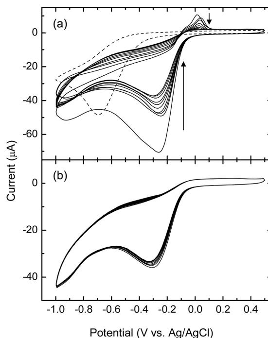
**Figure 3.** (a) First ten consecutive and (b) next ten consecutive cyclic voltammograms of pBpCuOx-coated GCE in 0.1 M acetate buffer (pH 4.7) saturated with O<sub>2</sub>. The dashed line was obtained on a bare GCE in the same solution. Scan rate = 100 mV·s<sup>-1</sup>.
