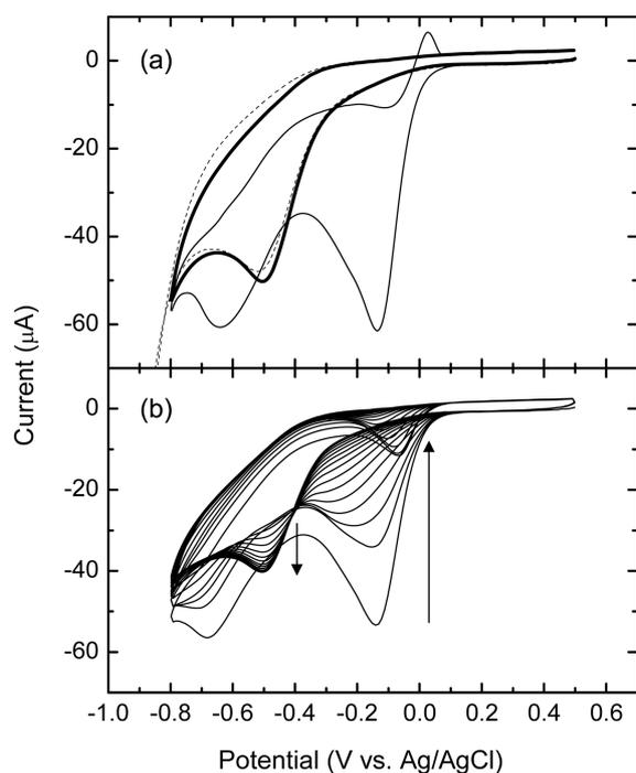
**Figure 4.** Cyclic voltammograms of pBpCuOx-coated GCE in 0.1 M H<sub>2</sub>SO<sub>4</sub> saturated with O<sub>2</sub>. (a) First (thin solid line) and seventeenth (thick solid line) cycles. (b) Consecutive cycles between second and sixteenth cycles. The dashed line was obtained on a bare GCE in the same solution. Scan rate = 100 mV·s<sup>-1</sup>.
