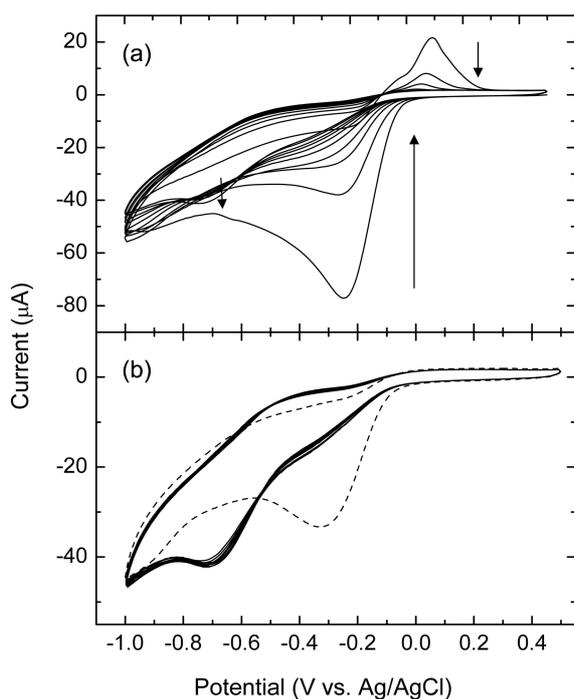
**Figure 8.** (a) First ten consecutive and (b) next ten consecutive cyclic voltammograms of BpCu-coated GCE in 0.1 M acetate buffer (pH 4.7) saturated with  $O_2$ . Dashed line was obtained on pBpCuOx-coated GCE in 0.1 M acetate buffer (pH 4.7) saturated  $O_2$  after 20 consecutive potential cycles. Scan rate =  $100 \text{ mV} \cdot \text{s}^{-1}$ .
