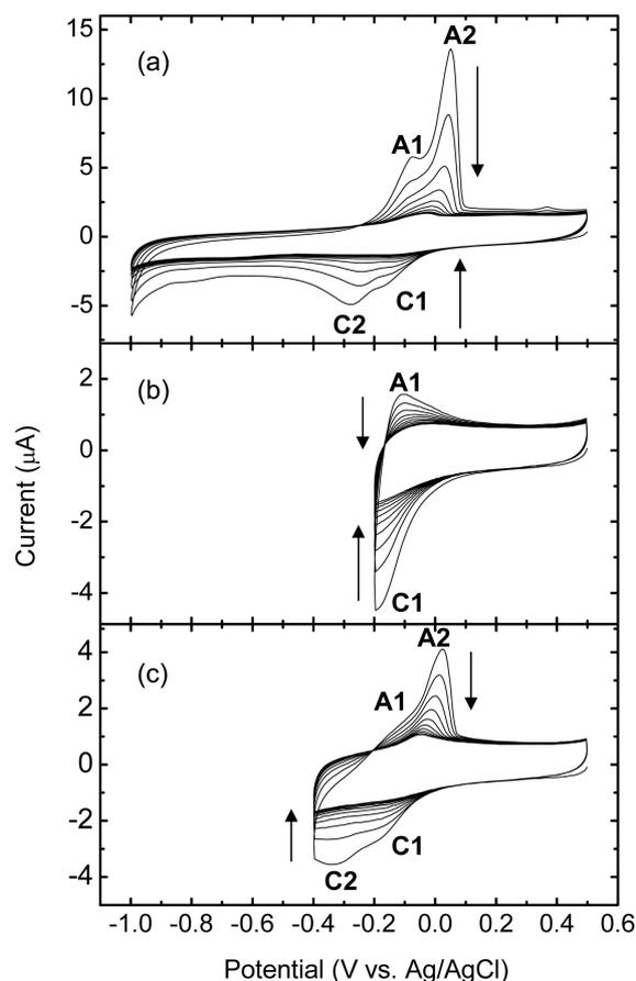
**Figure 2.** Ten consecutive cyclic voltammograms of pBpCuOx-coated GCE in 0.1 M acetate buffer (pH 4.7) saturated with Ar with a negative potential limit of (a)  $-1.0$  V, (b)  $-0.2$  V, and (c)  $-0.4$  V. Scan rate = 100  $mV \cdot s^{-1}$ .
