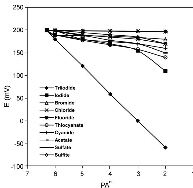
**Figure 2.** Potential responses of different ion-selective electrodes based on ICT.
