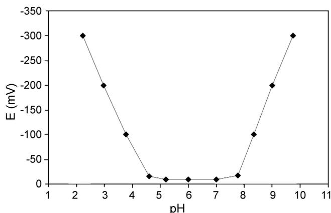
**Figure 5.** The effect of the pH of the test solutions on the potential response of the electrode based on ICT (No. 3).
