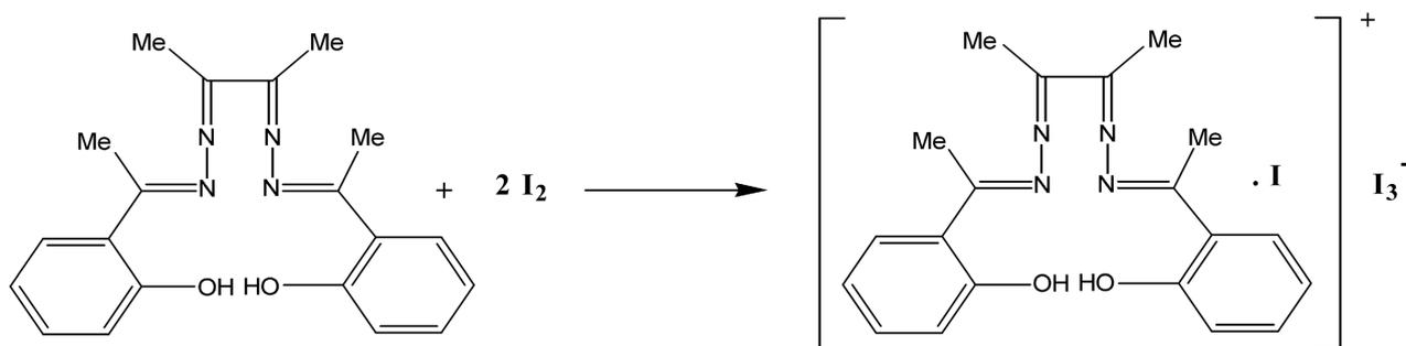
**Figure 1.** Chemical reaction of ICT preparation and chemical structure of ICT.
