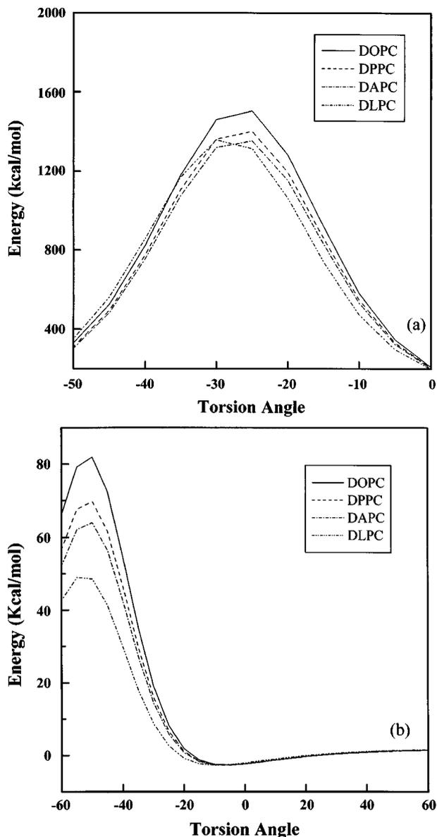
**Figure 6.** (a) Conformational energy curves of DOPC(C8), DPPC(C16), DAPC(C20), and DLPC(C24), (b) Interaction energy curve between two ( $\beta$ ,  $\gamma$ ) chains of DOPC(C8), DPPC(C16), DAPC(C20), and DLPC(C24) by CHARMM lipid force field.
