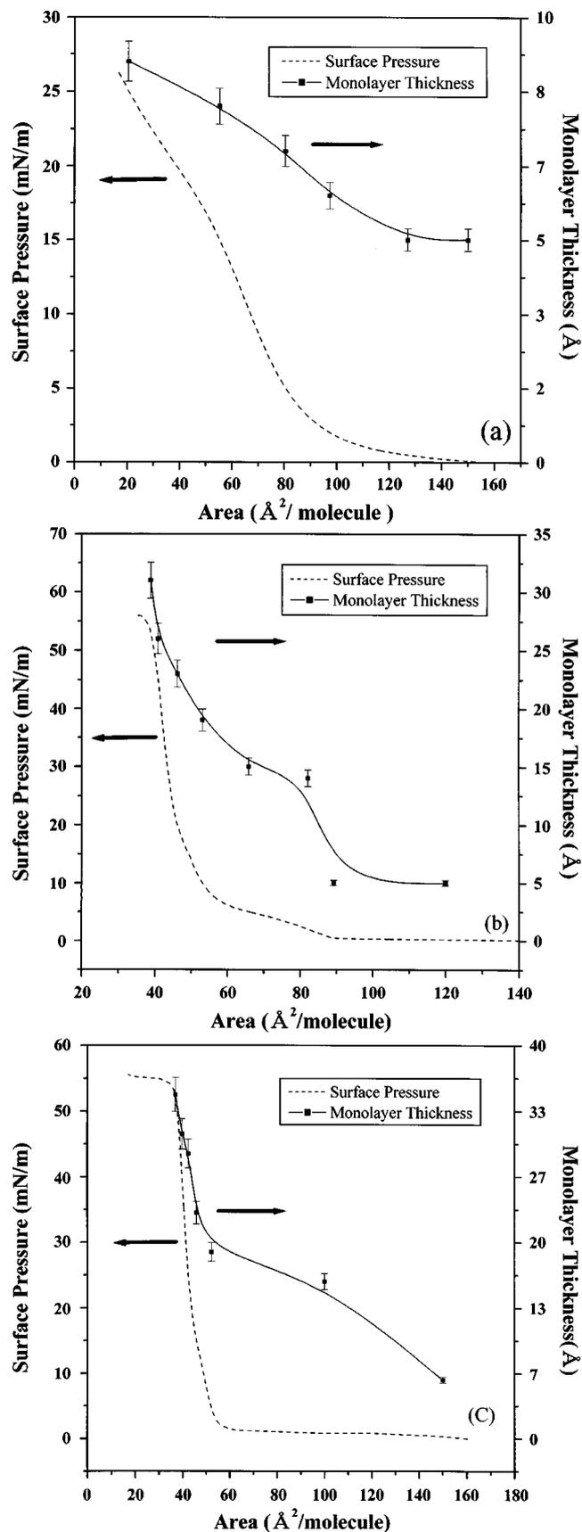
**Figure 3.** The  $\pi$ -A isotherms (—) and monolayer thickness vs. area per molecule ( $A_m$ ) curves (■) of (a) DOPC(C8), (b) DPPC(C16), and (c) DLPC(C24), at the air-water interface. The monolayer thickness was measured by ellipsometer.
