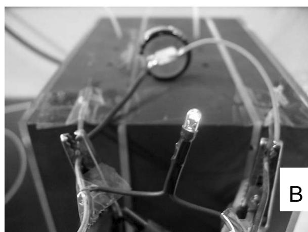
**Figure 7.** MFC output voltage change as a function of time (panel A) and the picture of powering of an electric bulb (panel B) from electricity stored in a 1 F supercapacitor.
