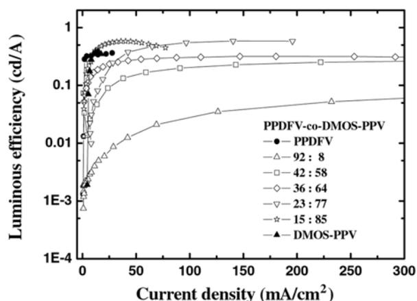
Figure 6. Efficiencies of PLEDs with a configuration of ITO/PEDOT/polymer/Al.
