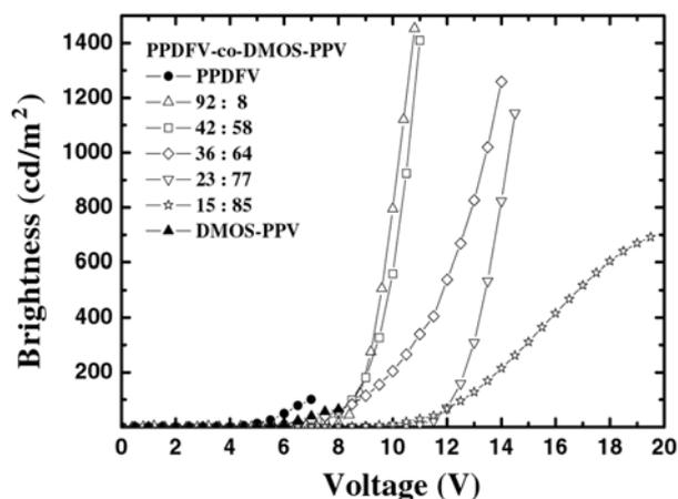
Figure 5. Luminescence-voltage ( $L$ - $V$ ) characteristics of ITO/PEDOT/polymer/Al devices.
