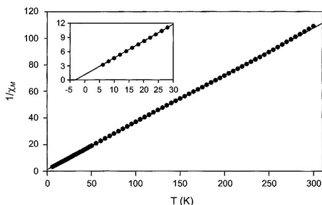
**Figure 4.** A plot of temperature against the reciprocal magnetic susceptibility of  $(\text{dmamth})_2\text{CoBr}_4$ .
