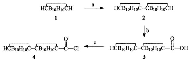
**Scheme 1.** (a) 1.2 eq of *n*-BuLi, 1.4 eq of anhydrous CuCl<sub>2</sub>, ether, 25 °C, 3 days, yield 40%. (b) 1 eq of *n*-BuLi, CO<sub>2</sub>, ether, 0-10 °C, 2h, yield 41%. (c) excess COCl<sub>2</sub>, Et<sub>3</sub>N, 90-100 °C, ortho-dichlorobenzene (*o*-DCB).
