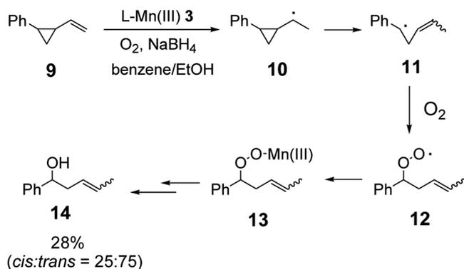
**Scheme 1.** Proposed mechanism for the oxygenation of vinylcyclopropane **9**.
